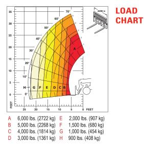
Load charts based on a 24" (610 mm) load center per ANSI/ITSDF B56.6
