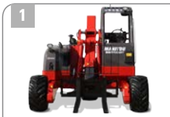
1 OPERATOR USES THE SIDESHIFT JOYSTICK TO CENTER THE BOOM.
