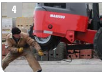
4 OPERATOR USES A HOOK TO EXTEND TWO SLIDE BARS TO SUPPORT THE WEIGHT OF THE MACHINE ON THE TRUCK.
