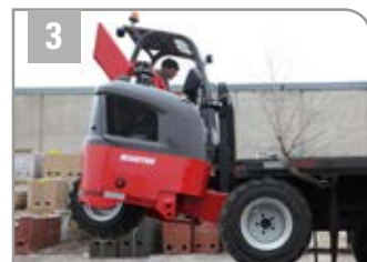
3 OPERATOR LOWERS THE BOOM AND TILTS UNIT FORWARD UNTIL FULLY ELEVATED.
