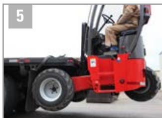
5 OPERATOR RETRACTS THE BOOM FULLY, RESTING THE TMT ON THE TWO SLIDE BARS, THEN TILTS MACHINE BACK ENSURING TIRES ARE FIRMLY AGAINST THE UNDERSIDE OF THE TRUCK BED.
