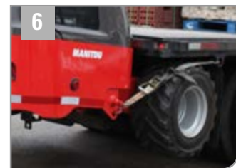
6 LASTLY, STRAPS ARE USED TO SECURE UNIT TO THE TRUCK BED.
