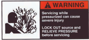
WARNING Servicing while pressurized can cause severe injury LOCK OUT source and RELIEVE PRESSURE before servicing PRESSURE RELIEF WARNING DECAL P/N 512572 FIGURE 1
